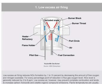
lower; flame length and stability can be negatively impacted.
